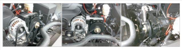
Alternator in a GMC with belt routing
